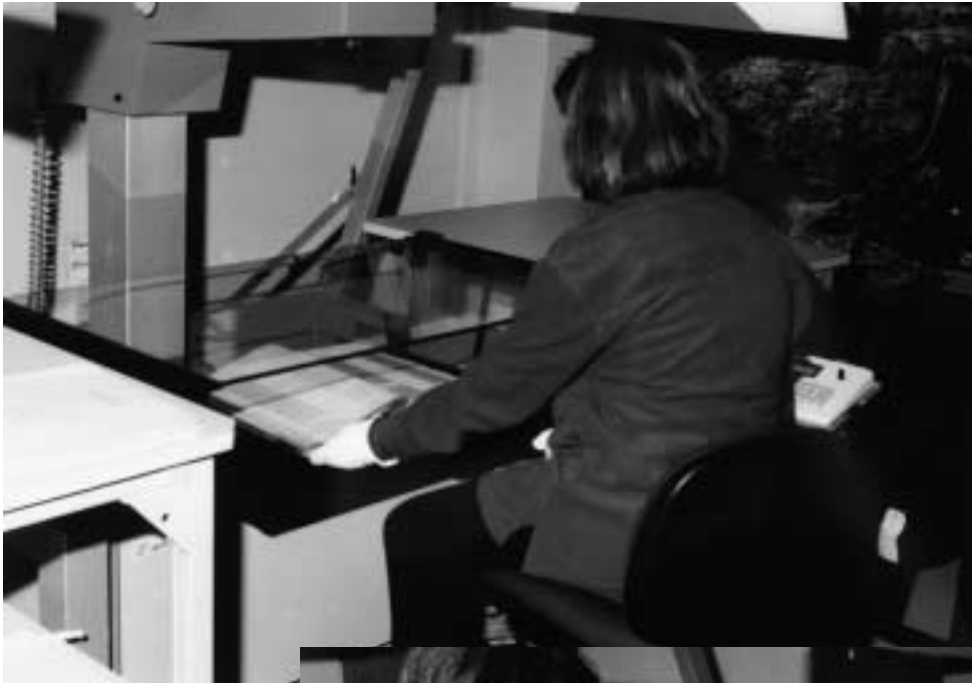
Camera with book lift and cradle in two operating positions
